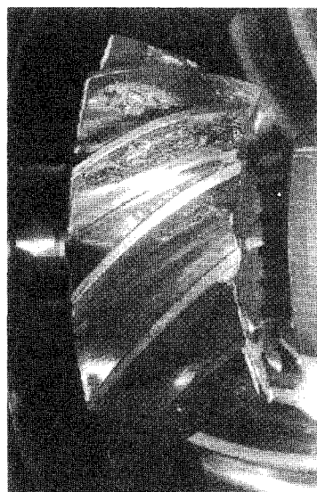
Fig. 6 Photograph of pinion damage at t = 14.53 h.
