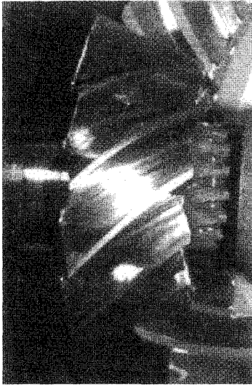
Fig. 1 Photograph of pinion at t = 5.50 h.
